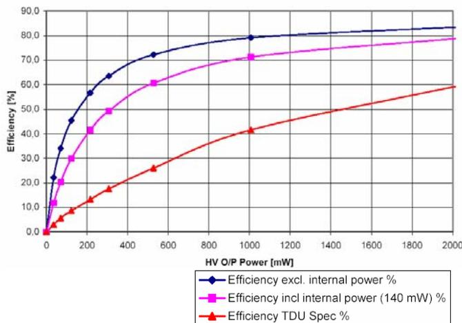
**Fig. 11: Efficiency of TDU Power Conditioning String vs. IE-Current @20V Bus Voltage (excluding internal power consumption -static value of approx. 140 mW)**
