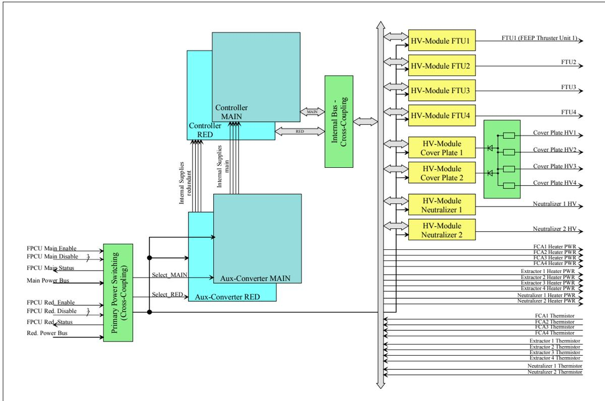
Fig. 11: Block Diagram of a FEEP Power Processing Unit
