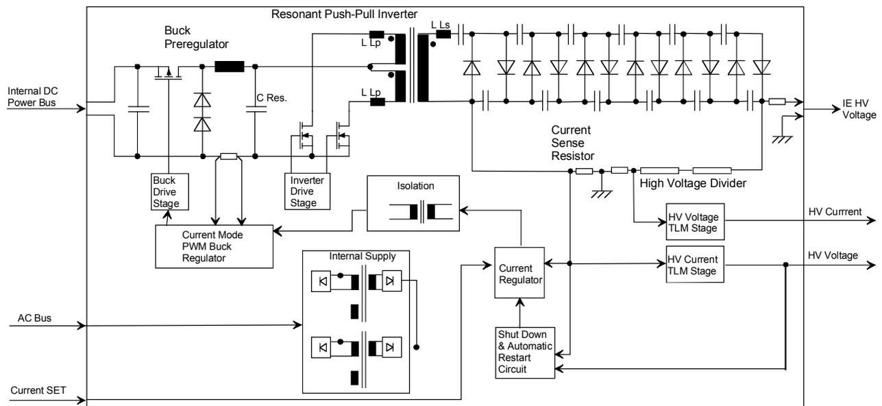
**Fig. 6: HVCV - High Voltage Converter Principle**
