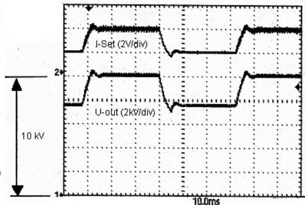
**Fig. 10: Step Response of Load Current (IE) and of Output Voltage (U-out) as a Result of Current Setting Step (I-Set) from 500  $\mu\text{A}$  to 1000  $\mu\text{A}$  - Time Scale: 10ms/div**
