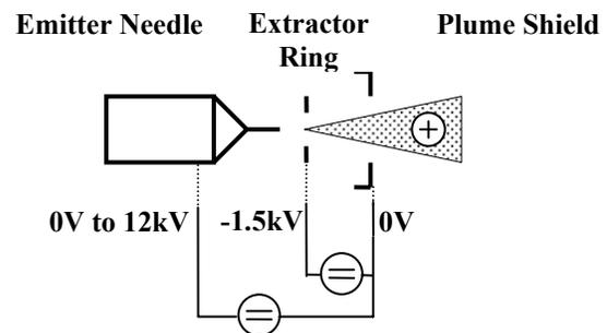
**Fig. 2: FEEP Ion Emitter (IE) Principle**
