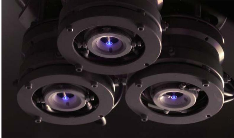
**Fig. 1: FEEP Microthruster Array under Test (Photo: Courtesy of ARCS Seibersdorf, Austria)**
