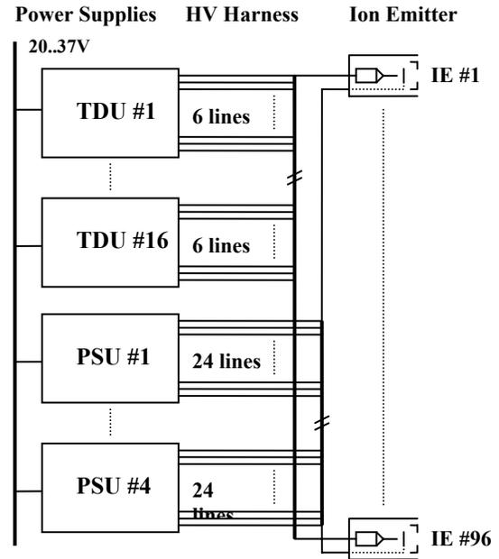
Fig. 3: FEPP Power System Units
