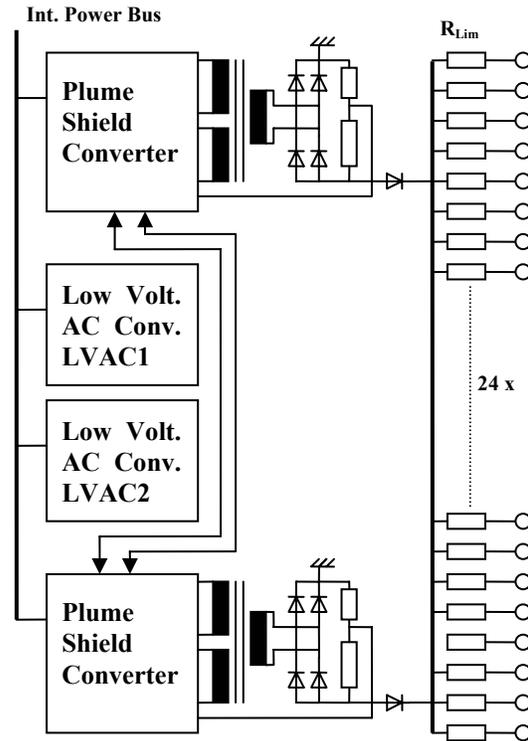
Fig. 7: Block Diagram of Plume Shield Unit
