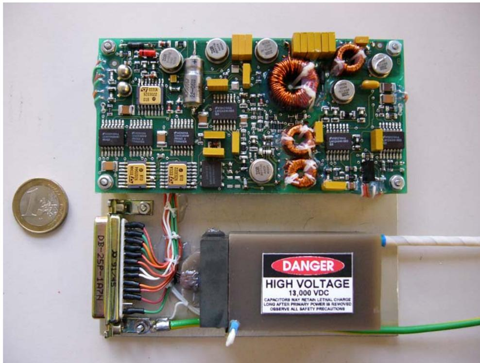
Fig. 9: Partial Breadboard Comprising a Low Voltage Converter (LVCV) and a High Voltage Converter (HVCV) with 13 kV High Voltage Module
