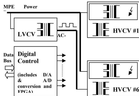
Fig. 4: TDU - Thruster Drive Unit Breakdown
