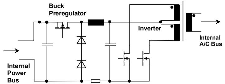
**Fig. 5: LVCV - Low Voltage Converter Principle**
