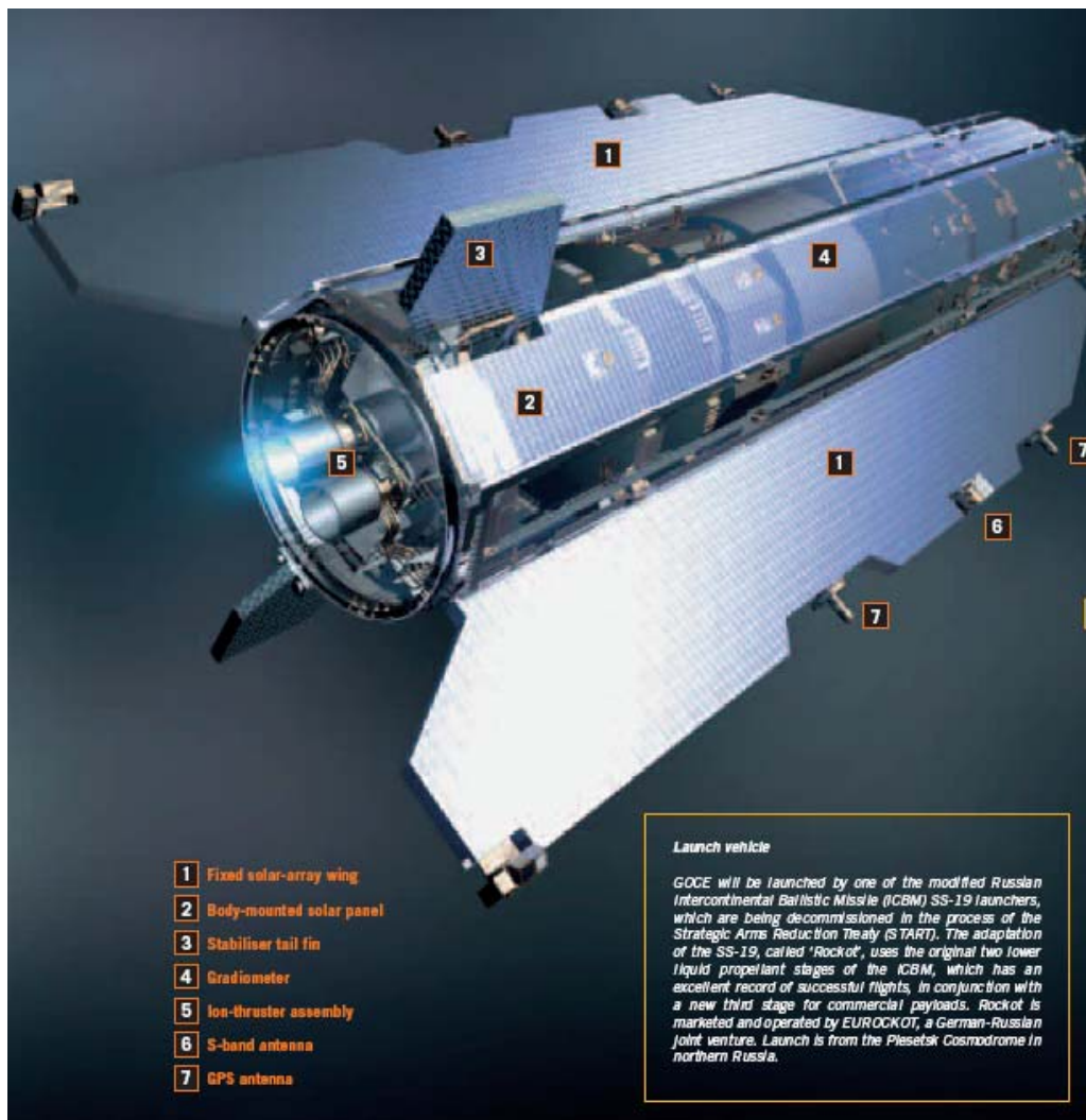
Fig. II-1: Spacecraft view, firing one of the redundant thrusters (Poster: ESA)
