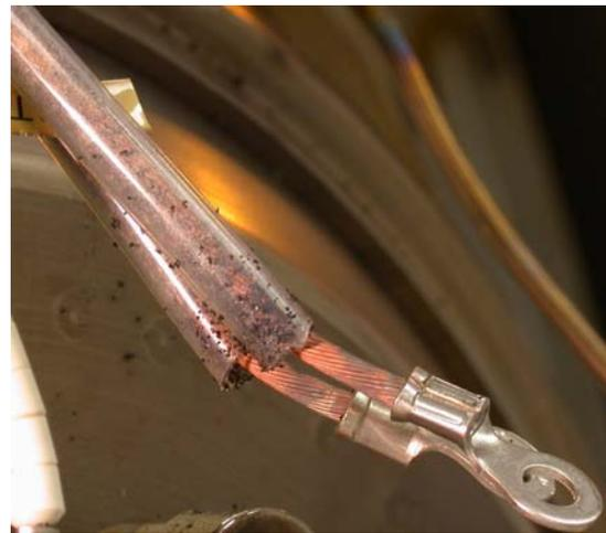
**Figure 17. Post-Test Inspection Photograph of Wire Harness Near Discharge Cathode Assembly. Note decomposition of wire insulation inside the intact Teflon sleeving.**
