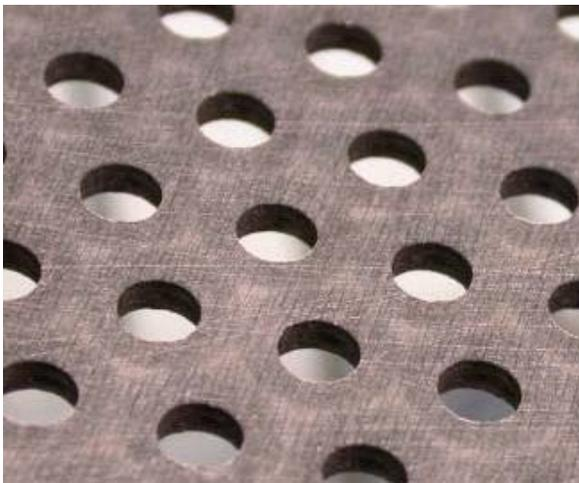
**Figure 16. Post-Test Inspection Photograph of Upstream Surface of Accelerator Grid. Note pristine, un-arc'd condition of surface.**
