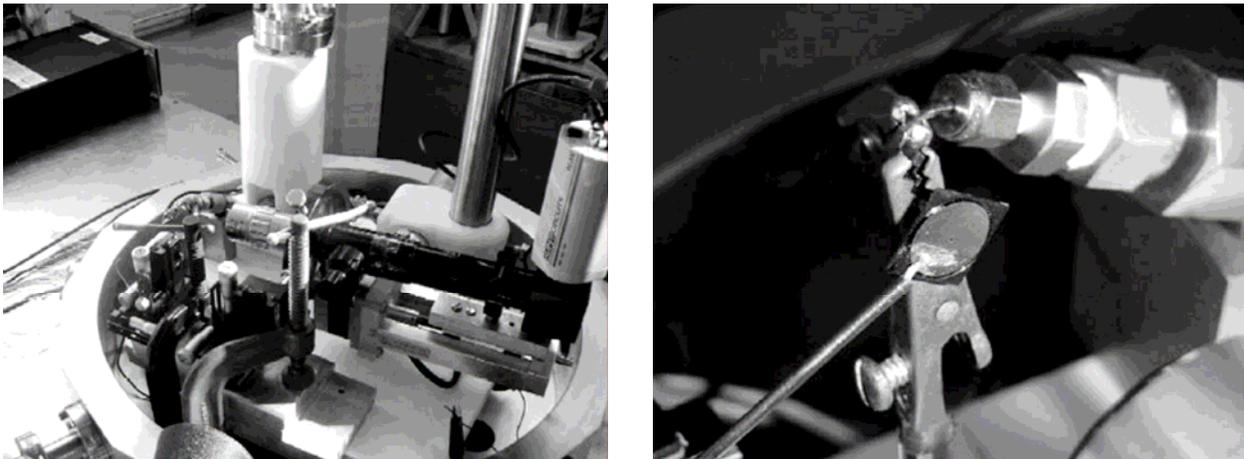
**Figure 3. Closeup of the microscope and emitter positioning stage (left), and a closeup of the emitter and attached electrode(right).**
