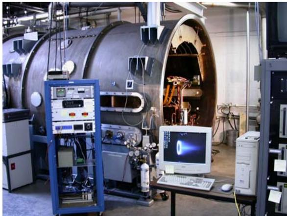
**Figure 2. Busek's 8-ft. diameter, 18-ft. long vacuum test facility**
