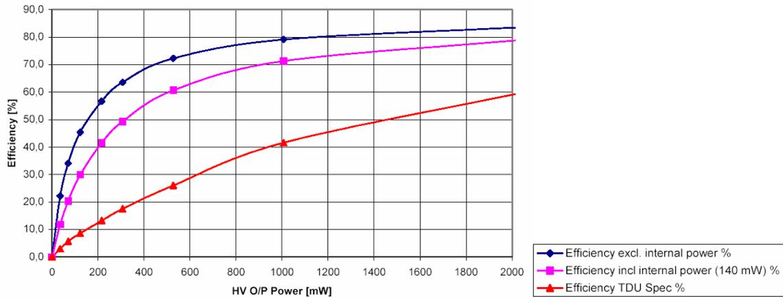
**Fig. 5: Efficiency of an Extractor Voltage Power Conditioning String vs. IE-Current @20V Bus Voltage (excluding internal power consumption -static value of approx. 140 mW)**
