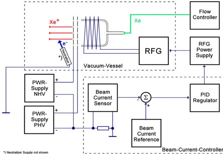
**Fig. 6: Block Diagram of a  $\mu$ -RIT Regulator Loop and Power Supplies**
