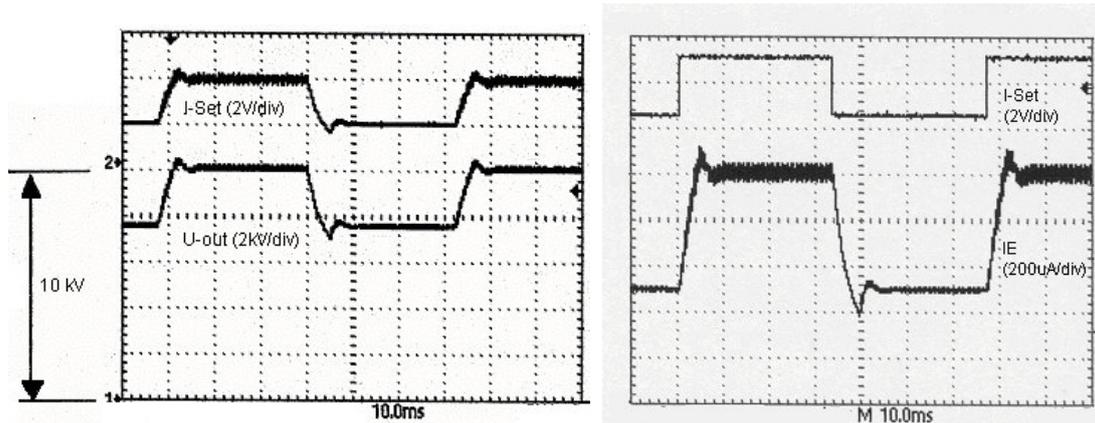
**Fig. 4: Step Response of Load Current (IE) and of Output Voltage (U-out) as a Result of Current Setting Step (I-Set) from 500µA to 1000µA - Time Scale: 10ms/div**
