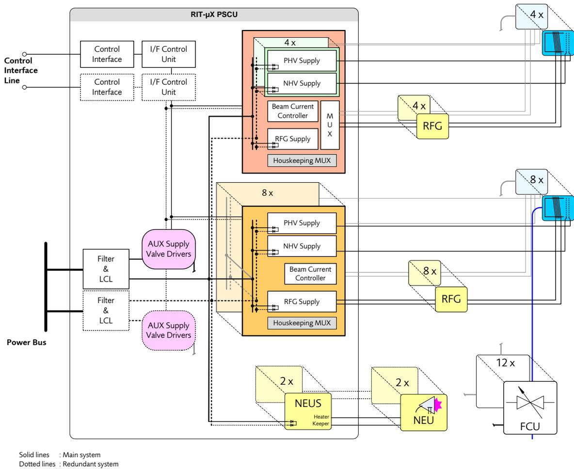
Fig. 7: Block Diagram of a  $\mu$ -RIT Power Supply & Control Unit for 12  $\mu$ -RIT thrusters
