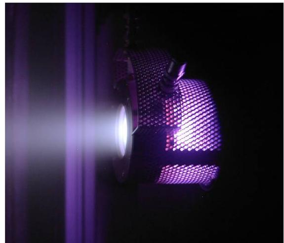
**Fig. 1: Firing of a  $\mu$ N-RIT**
