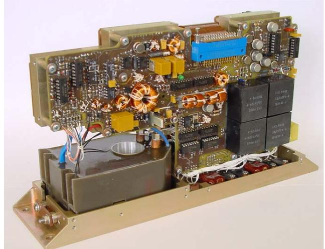
**Fig. III-5: High Voltage Power Supply Module (EM)**
