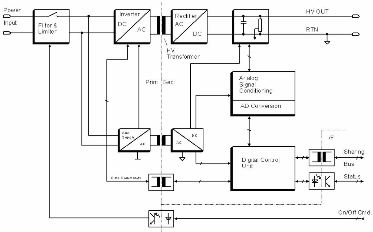
**Fig. III-2: Top-level Block Diagram of the Converter Module**
