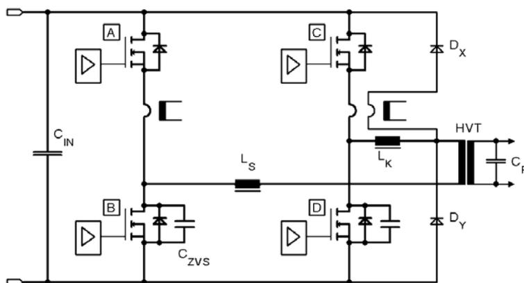
**Fig. III-3: Schematic of the Flattop-Converter for HVPS Next Generation**
