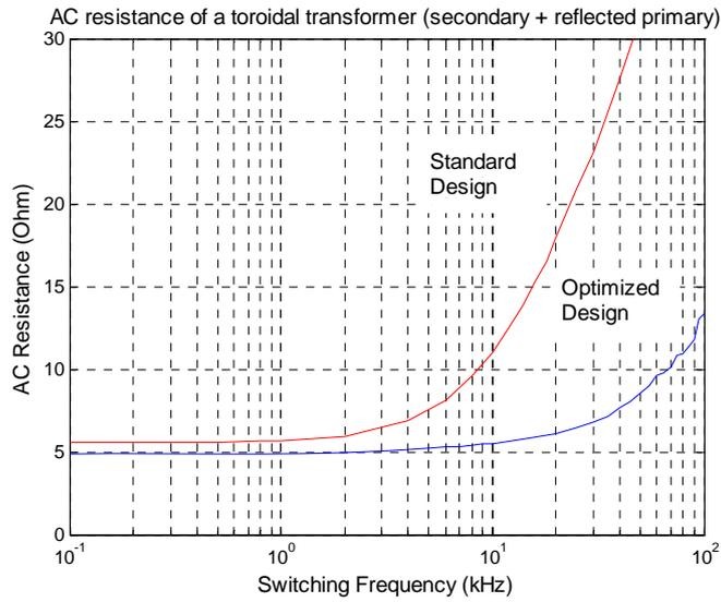
**Fig. III-4: Comparison of the proximity effect in terms of ac resistance of a hypothetical transformer**
