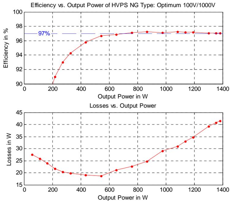
**Fig. III-6: Measured Efficiency of a the “Optimum” Module**
