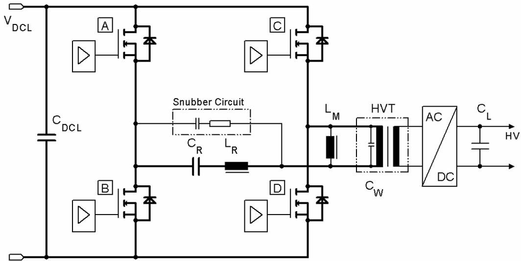
**Fig. IV-4: Block Diagram of the Resonant Converter Stage**
