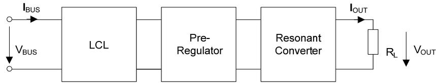
**Fig. IV-1: Two Stage Concept with Pre-Regulator followed by an Resonant Converter**
