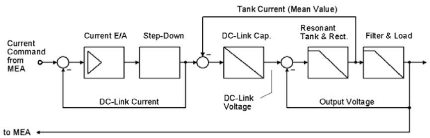
**Fig. IV-2: Cycle Based Averaged Model of the Step-down and Resonant stage**
