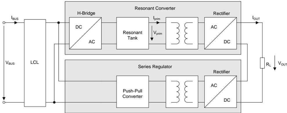
**Fig. IV-3: Block Diagram DC-Output Series Connected Converter**
