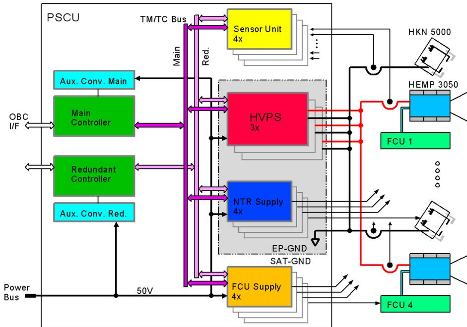
**Fig. V-1: Power Supply Control Unit (= Power Processing Unit) for HEMP Thruster Unit**
