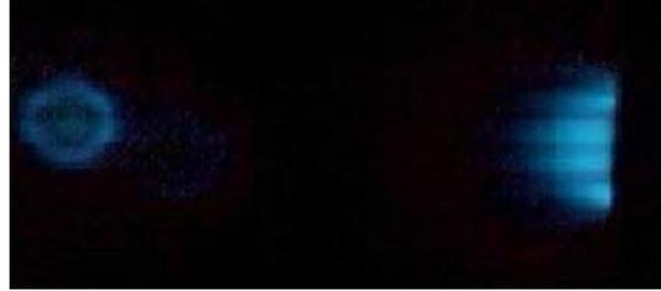
Figure 6. Luminescence (suppressed) of plasma while SPT M-70 operated in mode: discharge voltage  $U_d=70$  V, magnetic induction on discharge chamber edge  $B=16$  mTl.
