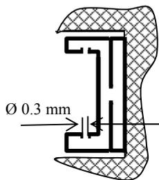
**Figure 3. The scheme of the SPT anode – gas distributor with separate radial apertures.**
