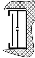
**Figure 9. The scheme of the anode-gas distributor with the separate apertures (10 mm distance) closed by deflector.**
