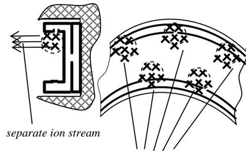
Areas of intensive ionization of gas close to the separate apertures in the anode – gas distributor.
