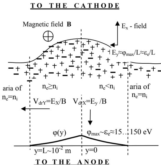
Figure 8. Possible polarization of plasma charges in the area of non-uniform concentration – seen as area of the increased intensity of plasma luminescence.
