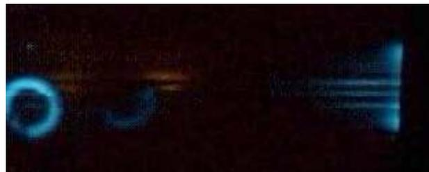
**Figure 4. Luminescence (suppressed) of plasma while SPT M-70 operated in mode: discharge voltage  $U_d=250$  V, magnetic induction on discharge chamber edge  $B=16$  mTl.**
