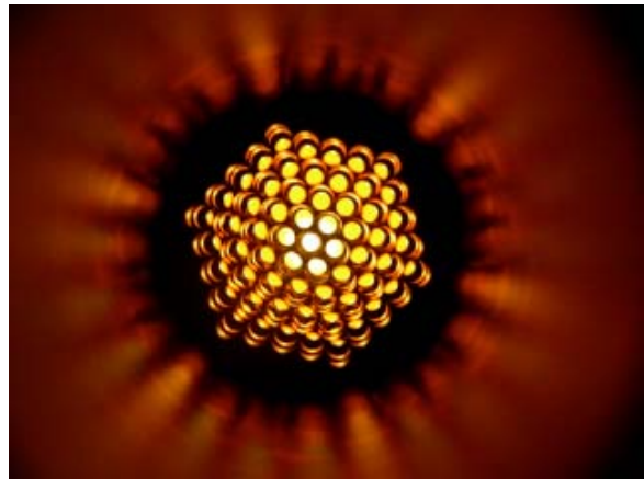
Figure 4. Thruster screen grid with open area ratio of 61%.
