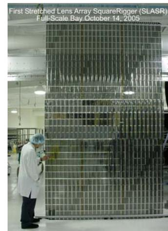
**Figure 2. Full scale SLASR panel**
