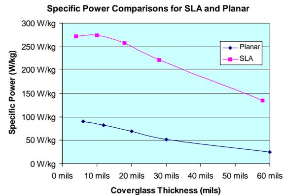
Figure 8. Specific power comparison for SLA and Planar Arrays
