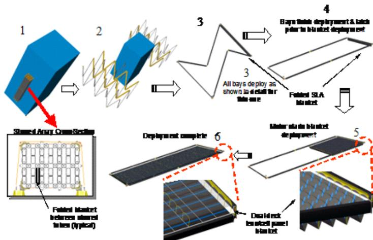
**Figure 3. Stretched Lens Array SquareRigger Deployment**
