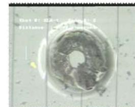
**Figure 5. Lens sample after hypervelocity test**
