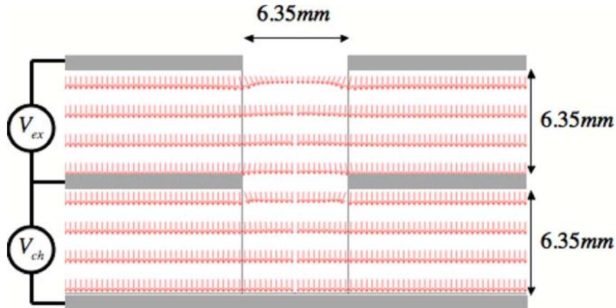
**Figure 16: Simulation showing direction of electric field in multi-grid structure when using ratio of electrode gap to channel diameter of one.**
