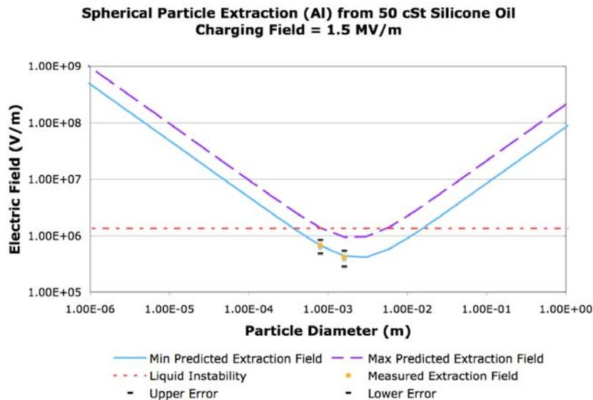
**Figure 10: Plot of the theoretical threshold extraction and threshold instability electric fields when extracting aluminum spherical particles from 50 cSt silicone oil using a charging electric field of 1.5 MV/m along with experimental results.**
