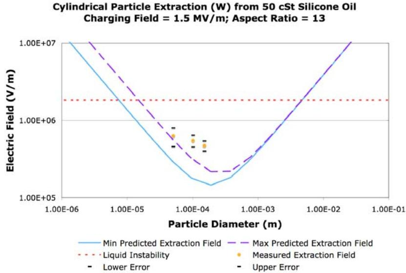
**Figure 13: Plot of the expected threshold extraction and threshold instability electric fields when extracting tungsten cylindrical particles with an aspect ratio of 13 from 50 cSt silicone oil using a charging electric field of 1.5 MV/m along with experimental results.**
