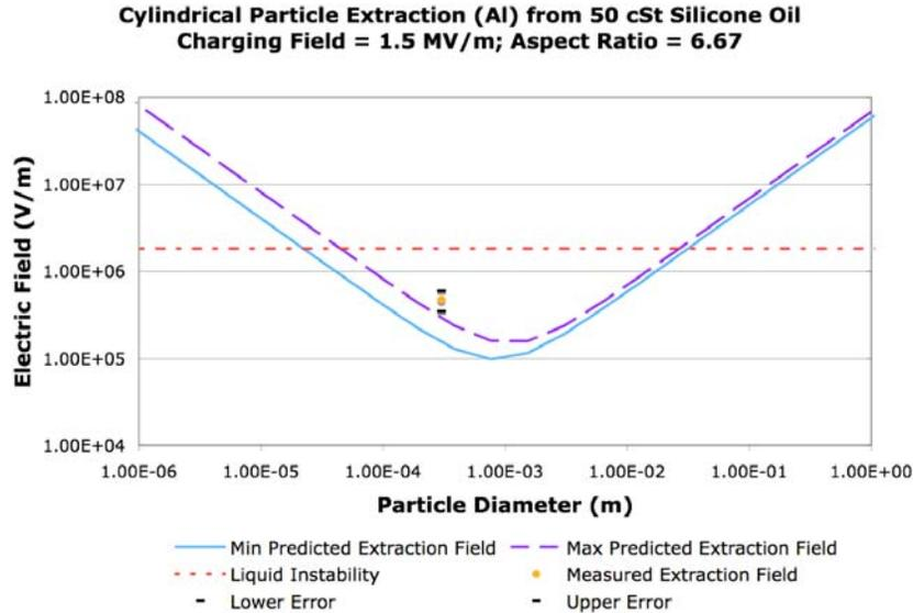
**Figure 12: Plot of the expected threshold extraction and threshold instability electric fields when extracting aluminum cylindrical particles with an aspect ratio of 6.67 from 50 cSt silicone oil using a charging electric field of 1.5 MV/m along with experimental results.**
