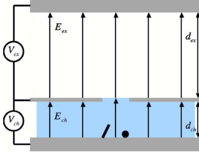
**Figure 7: Experimental setup for particle extraction from insulating liquid when decoupling the charging and extraction electric fields.**
