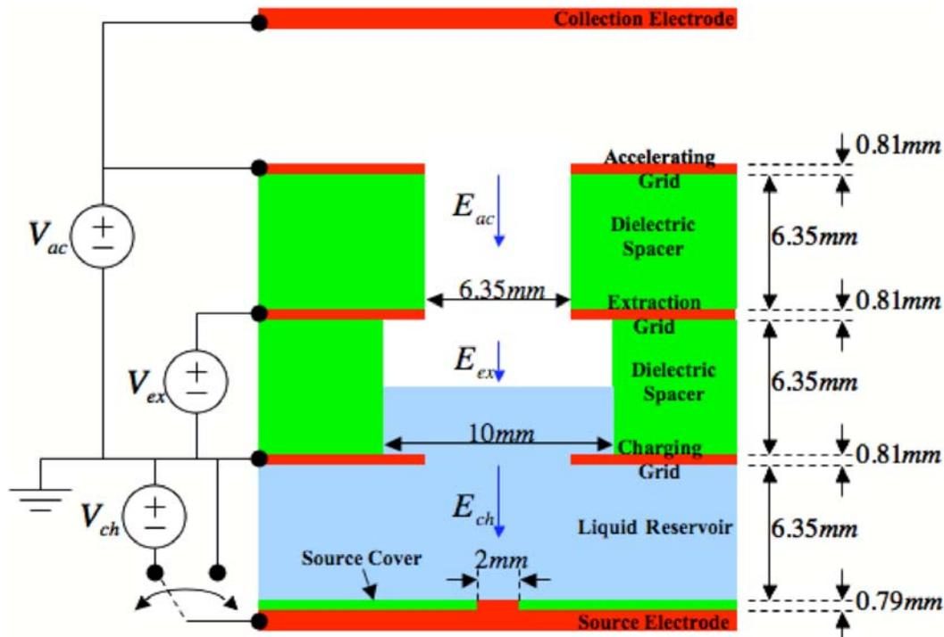
Figure 17: schematic showing the cross-sectional view of a single emitter for a future generation prototype with liquid surface between charging and extraction grids to reduce radial electric fields at extraction point.
