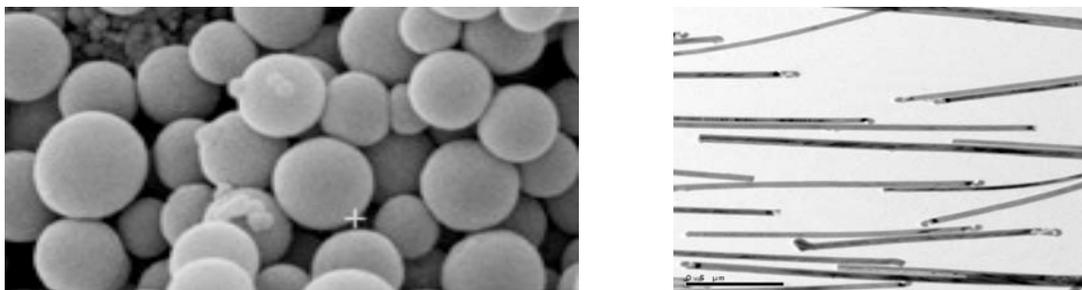
Figure 2: Example of a collection of unsorted nanoparticle spheres in the 10 nm diameter range (left) and cylinders with a diameter of 45  $\mu\text{m}$  and length of 500  $\mu\text{m}$ .
