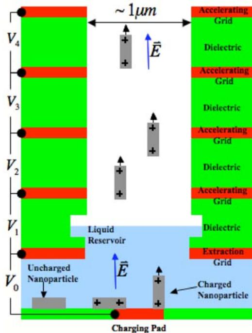
Figure 3: Cross-section schematic of a single emission channel used in the microparticle emitter prototype.
