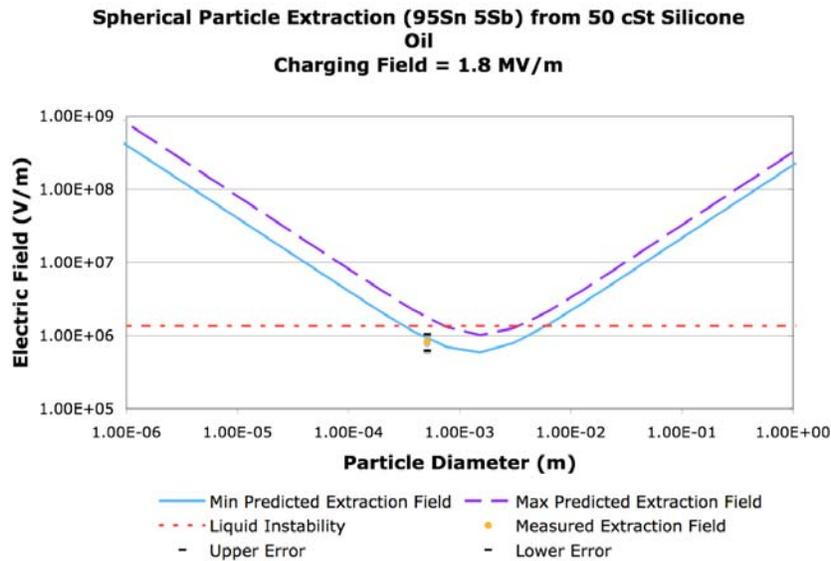
**Figure 11: Plot of the expected threshold extraction and threshold instability electric fields when extracting 95Sn/5Sb spherical particles from 50 cSt silicone oil using a charging electric field of 1.8 MV/m along with experimental results.**
