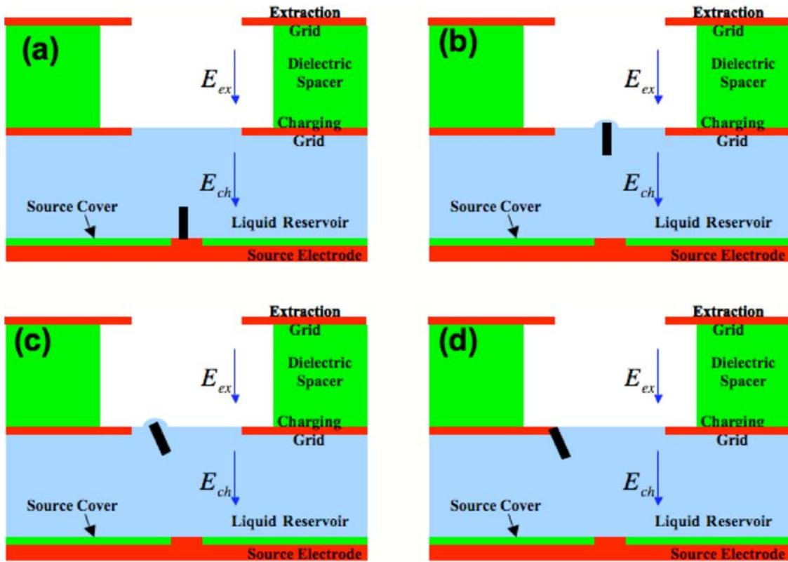
Figure 15: Typical progression of an unsuccessfully extracted cylindrical particle. (a): Particle is charged on exposed source electrode. (b): Particle transported to liquid surface and decelerated by surface tension. (c): Radial electric fields rotate particle and pull it towards charging grid. (d): Particle crashes into charging grid and undergoes a charge exchange to end possibility of particle extraction.
