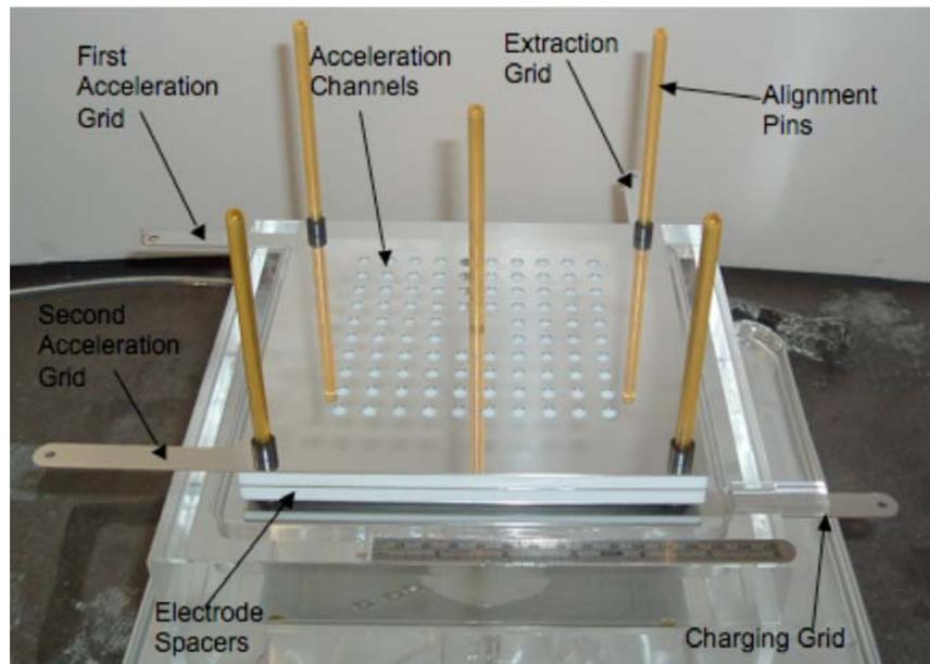
**Figure 9:** Picture of the first generation microparticle emitter prototype used to charge, extract, accelerate, and eject micron sized particles.
