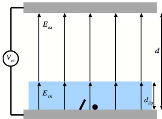
Figure 6: Experimental setup for particle extraction from an insulating liquid using a dual electrode extractor.
