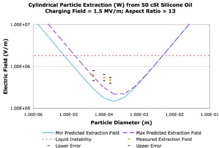
**Figure 14: Plot of the expected threshold extraction and threshold instability electric fields when extracting tungsten cylindrical particles with an aspect ratio of 60 from 50 cSt silicone oil using a charging electric field of 1.5 MV/m along with experimental results.**
