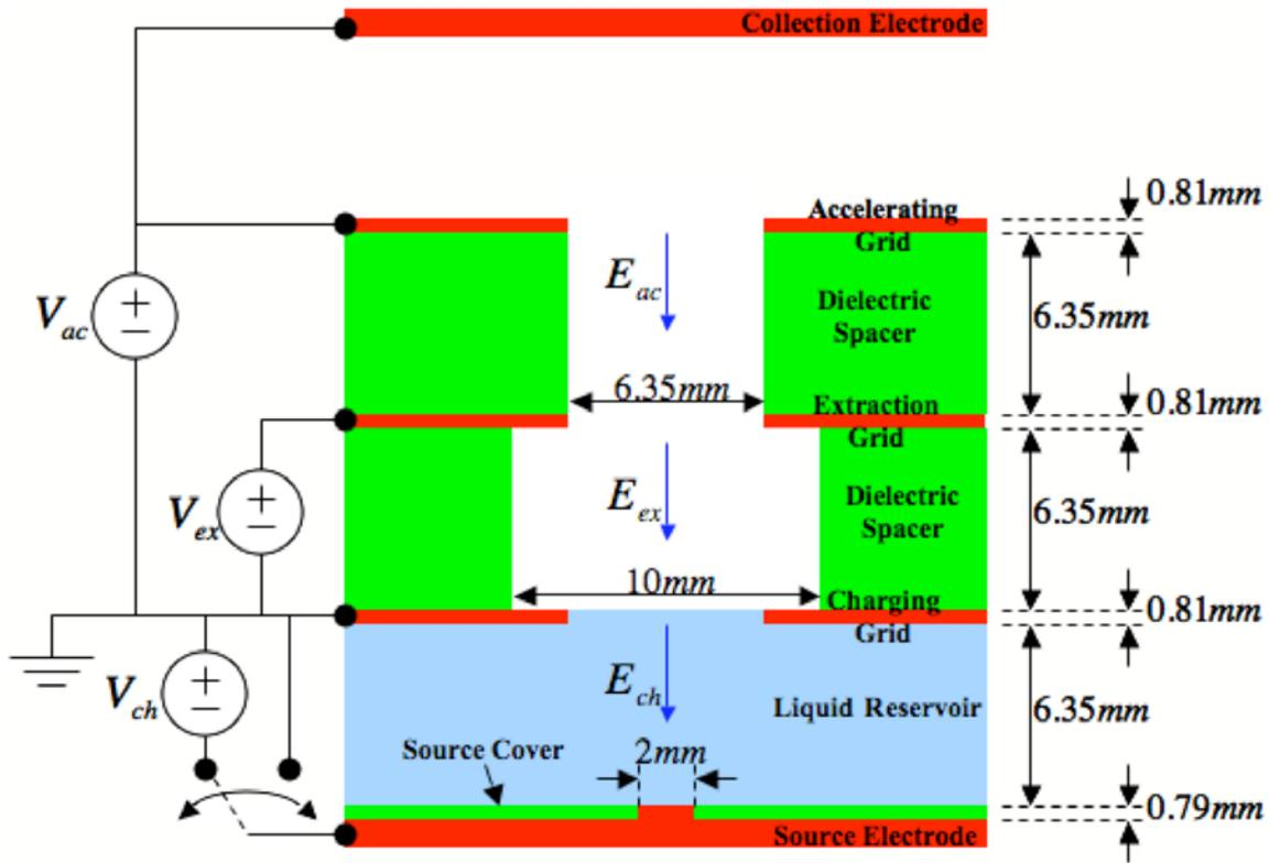
Figure 8: Schematic showing the cross-sectional view of a single emitter used in the first generation microparticle emitter prototype.
