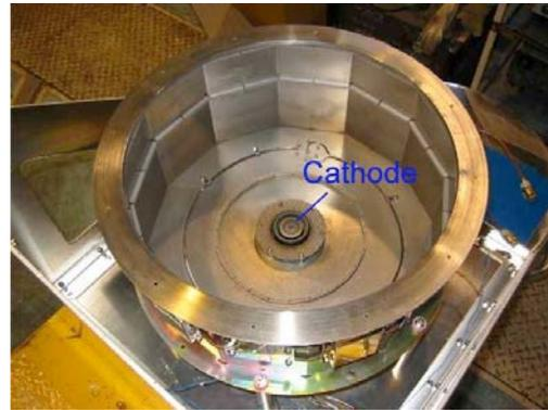
**Figure 3. Discharge chamber for life test.**
