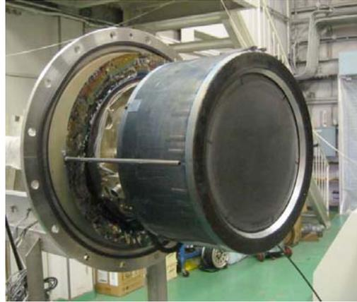
**Figure 1. Breadboard model of JAXA next-generation ion engine.**
