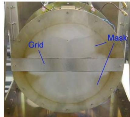
**Figure 4. Grid and mask on discharge chamber.**
