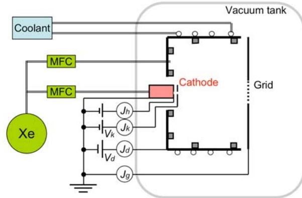
Figure 5. Configuration of life test.
