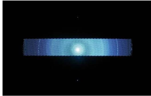
**Figure 7. Discharge luminescence through masked grid.**
