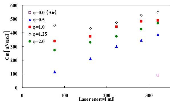
Fig.7 Variations of momentum coupling coefficient with laser-pulse energy for various equivalence ratios measured by thrust stand for conical nozzle with the half-cone angle of 7.5 deg.
