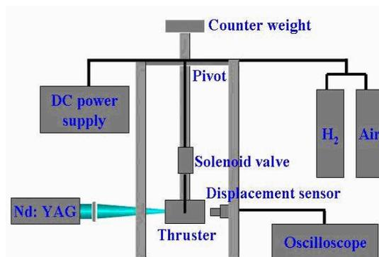
Fig.2 Schematics of pendulum-type thrust stand and experiment setup of impulse-bit measurement.
