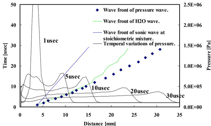
Fig.11 Temporal evolutions of shockwave and reacting wave fronts for laser energy of 167 mJ for half-cone angle of 15 deg. and stoichiometric mixture of  $\phi = 1.0$ .
