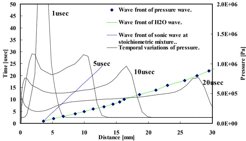
Fig.12 Temporal evolutions of shockwave and reacting wave fronts for laser energy of 167 mJ for half-cone angle of 7.5 deg. and stoichiometric mixture of  $\phi = 1.0$ .
