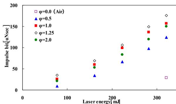
Fig.5 Variations of impulse bit with laser-pulse energy for various equivalence ratios measured by thrust stand for a conical nozzle with half-cone angle of 7.5 deg.
