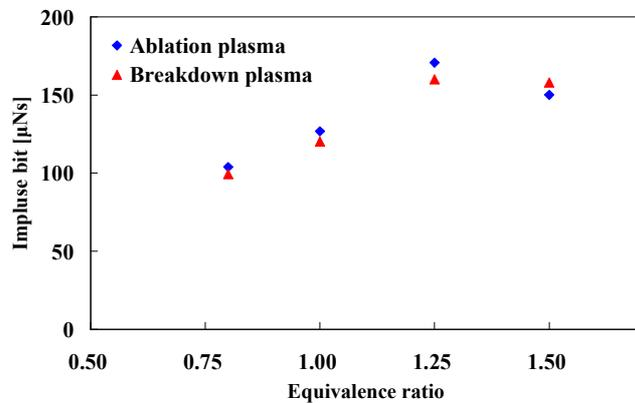
Fig.8 Relations of impulse-bit versus equivalence ratio for laser ablation plasma and breakdown plasma for a nozzles with half-cone angle of 15 deg., laser energy of 275 mJ.
