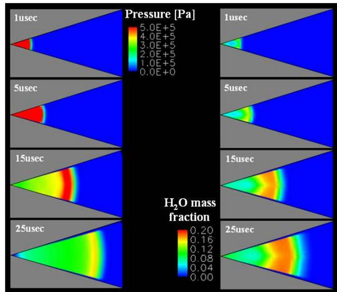
Fig.10 Temporal evolutions of propagation of pressure wave and H<sub>2</sub>O mass fraction distribution for laser energy of 167 mJ for half-cone angle of 15 deg. and stoichiometric mixture of  $\phi = 1.0$ .
