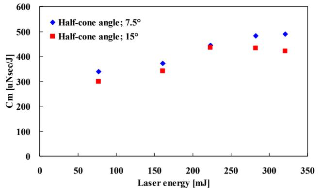
Fig.4 Comparison of momentum coupling coefficient versus laser-pulse energy for nozzles with half-cone angle of 7.5 deg. and 15 deg. for stoichiometric mixture of  $\phi = 1.0$ .
