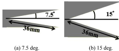
Fig.1 Schematics of conical-nozzle thrusters with different half-cone angles.
