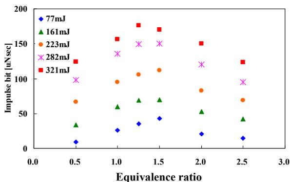
Fig.6 Variations of impulse bit with equivalence ratio for various laser-pulse energies measured by thrust stand for a conical nozzle with half-cone angle of 7.5 deg.
