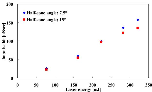
Fig.3 Comparison of impulse-bit versus laser-pulse energy for nozzles with half-cone angle of 7.5 deg. and 15 deg. for stoichiometric mixture of  $\phi = 1.0$ .
