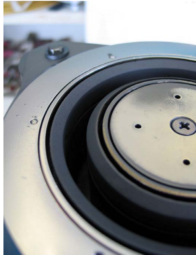
Figure 34. After erosion testing, 6 o'clock, camera location 3 o'clock.
