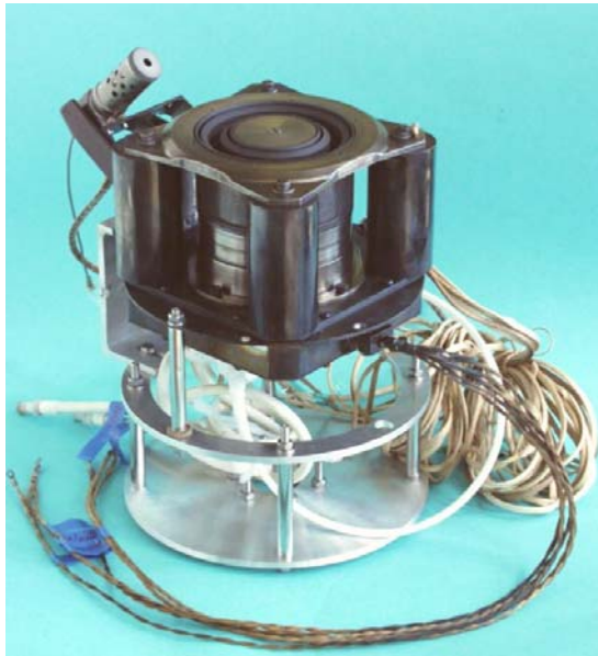
Figure 2. D-80 prepared for testing at EDB "FAKEL" facility.
