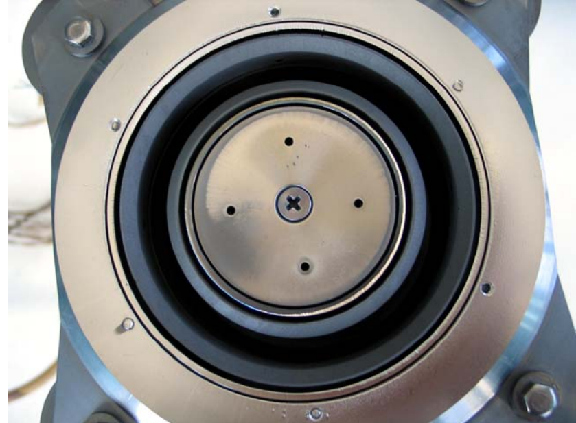
Figure 28. After erosion testing, top view.
