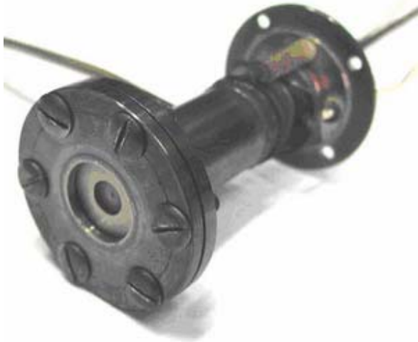
Figure 1. Cathode mock-up with disassemble diaphragm.
