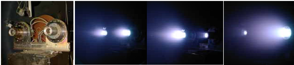
Figure 1.9. Two HEMP 3050 thrusters mounted on a horizontal bar in 40 cm distance on top of the thrust balance. Thrusters are operating on one anode supply line at 1000V, individual thruster adjustments by Xe flow to: 2x 2 kW, 2 kW + 300 W and 300 W+ 2 kW (from left to right)
