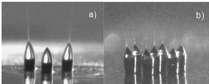
**Figure 1. CCD images of cone-jet structures formed on a micro-fabricated a) 3 emitter array and b) 7 emitter array from Ref 2**
