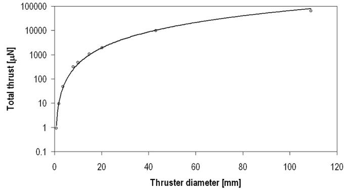
Figure 8. Thruster diameter scaling
