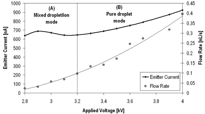
Figure 4. Emitter current and flow rate vs applied voltage for EMI BF<sub>4</sub>.
