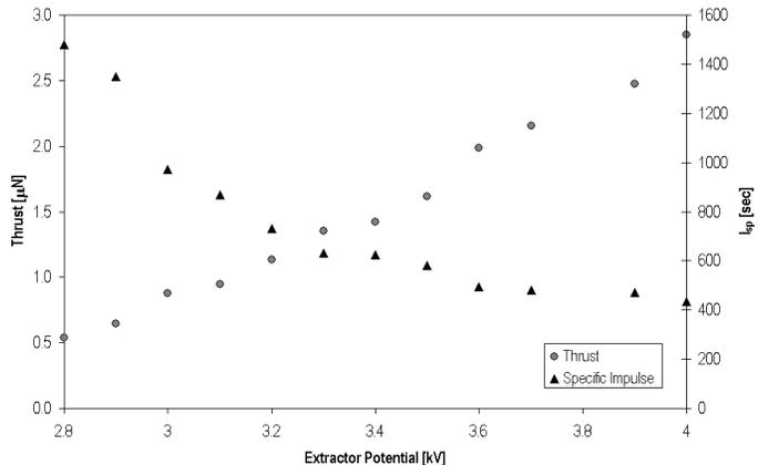
Figure 5. Effect of extractor voltage on Thrust and Specific Impulse
