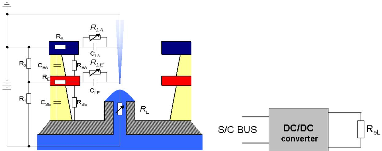
Figure 9. a. Circuit diagram of colloid thruster nozzle
