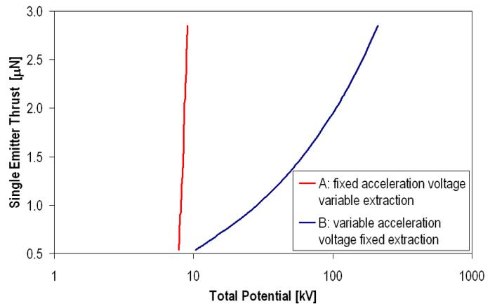
Figure 6. Required Potentials for Thrust Throttling
