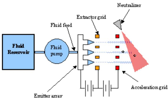
**Figure 2. Schematic of a conventional colloid thruster system**
