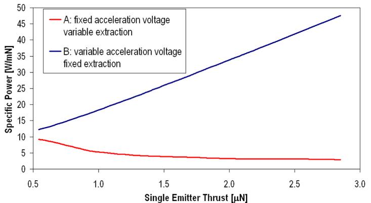
Figure 7. Effect of Thrust Throttling on Specific Power
