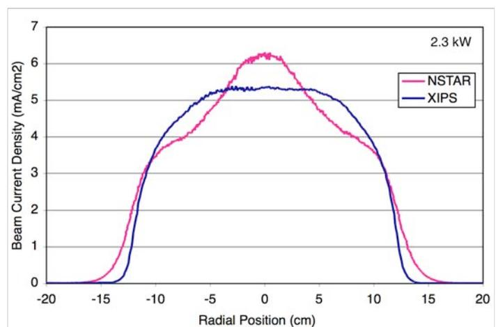
**Figure 13. Comparison of the beam profiles of XIPS and NSTAR at the 2.3 kW thruster input power point.**
