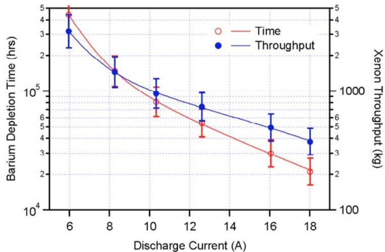
**Figure 4. Barium depletion time calculated for the XIPS discharge hollow cathode as a function of discharge current level showing extensive cathode life.**
