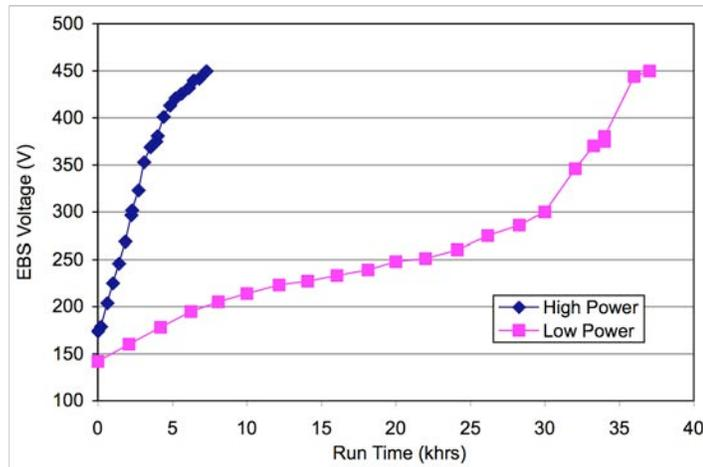
**Figure 12. Magnitude of the voltage at which electron backstreaming occurs as a function of time for each of the XIPS high power and low power cases.**
