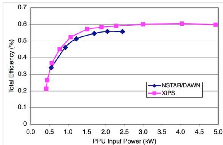
Figure 2. Total efficiency of the 25-cm XIPS thruster and PPU and the NSTAR thruster and PPU as used on DAWN versus PPU input power.
