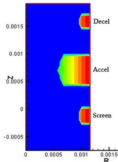
**Figure 7. Initial conditions of the XIPS grids input into the CEX-2D code.**
