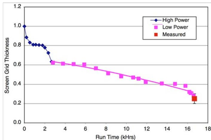
**Figure 11. Mean screen grid thickness calculated during the 25-cm XIPS thruster life test and the measured end point.**
