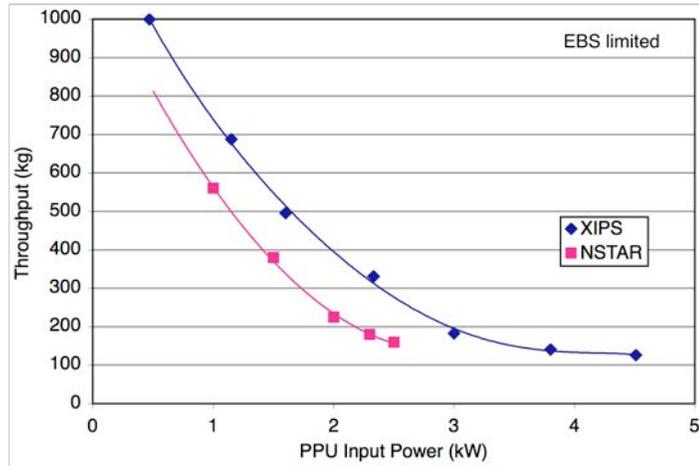
**Figure 14. Maximum engine throughput for XIPS and NSTAR, limited by electron backstreaming, as a function of PPU in put power.**
