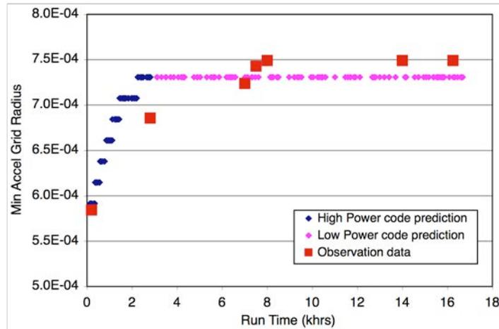
**Figure 10. Predicted and observed minimum accel grid hole diameter during the 25-cm XIPS thruster life test.**
