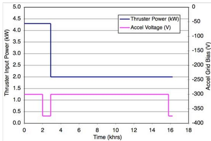
**Figure 6. Thruster input power level and accel grid bias voltage during the 25-cm XIPS thruster life test.**
