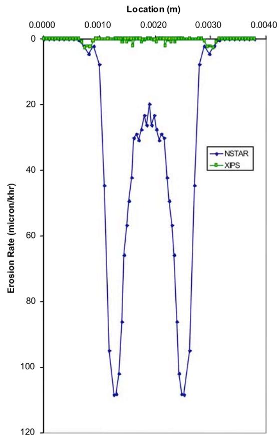
**Figure 5. Calculated Pits and Grooves erosion rates<sup>12</sup> showing the XIPS 3<sup>rd</sup> grid effectiveness compared to the 2-grid NSTAR erosion rate.**
