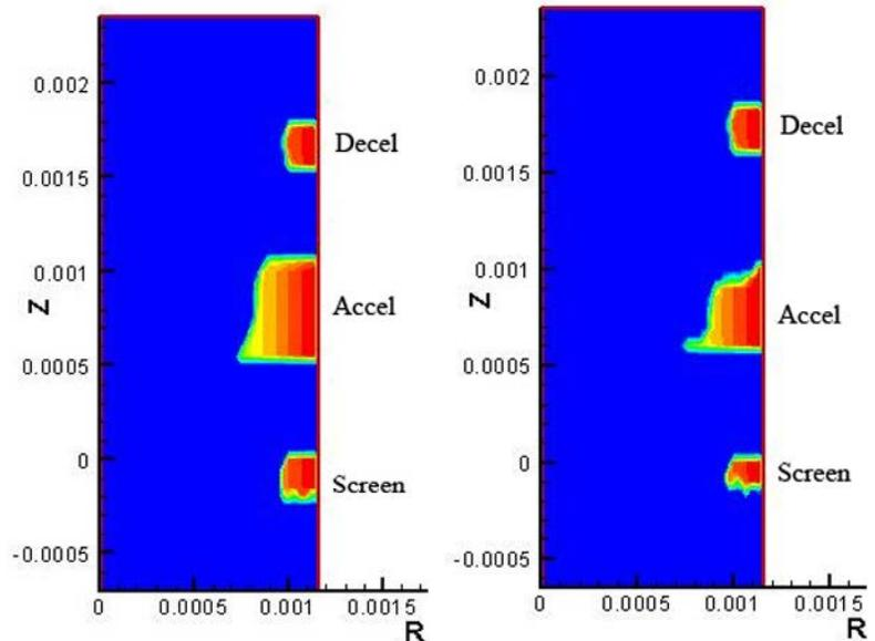
**Figure 8. Eroded grids at 2.8 khrs (left) at the end of the high power mode operation and 16.8 khrs (right) at the end of the low power mode operation.**
