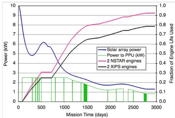
**Figure 15. Maximum engine throughput for XIPS and NSTAR, limited by electron backstreaming, as a function of PPU input power.**
