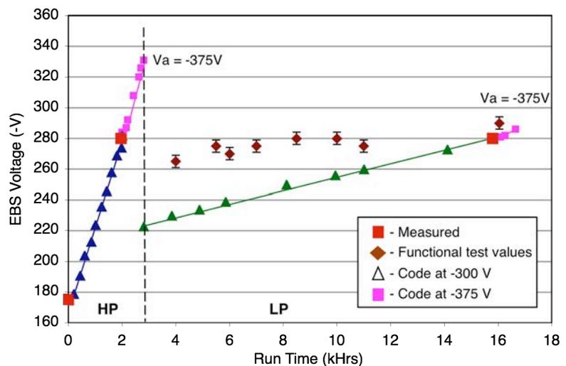
**Figure 9. Measured and calculated electron backstreaming voltage during the 25-cm XIPS thruster life test.**
