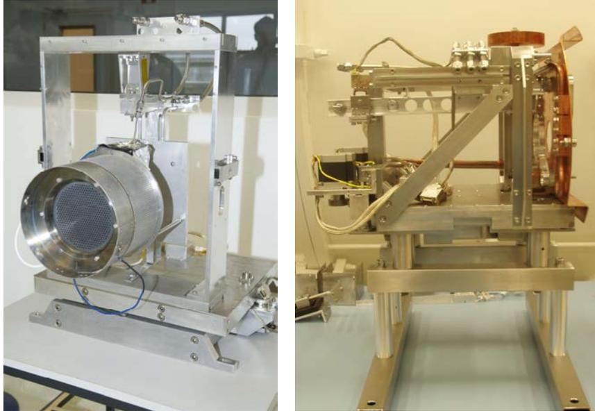
Figure 4. a) 1-axis optical thrust stand with GIS-15 and b) Low thrust balance
