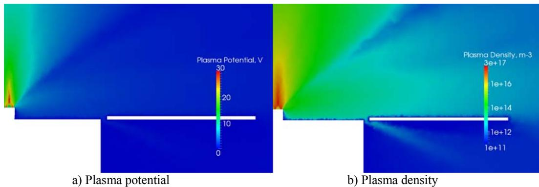
Figure 10. Plasma potential and electron number density
