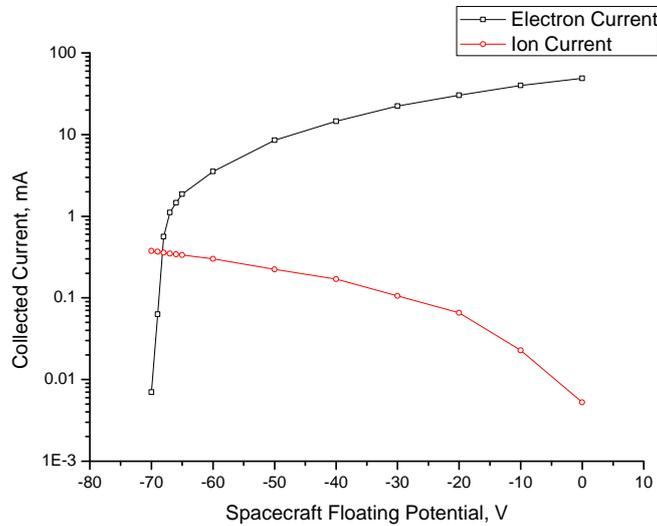
**Figure 12. Current collection according to spacecraft floating potential**
