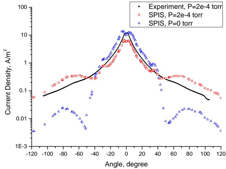
**Figure 6. Comparison of current densities at sweep radius 0.37m**
