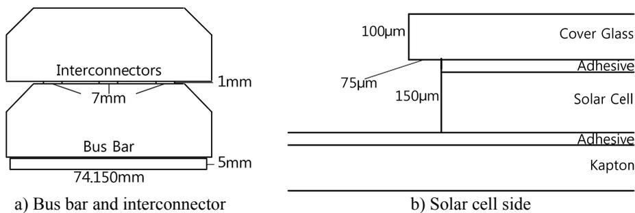
**Figure 3. Current collectors, both sides of interconnectors are exposed**
