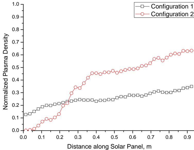
**Figure 16. Plasma density along solar panel, normalized by no shield result**
