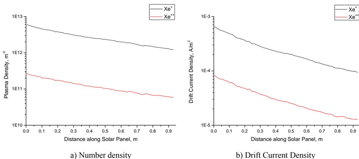
Figure 11. Plasma properties along the solar panel
