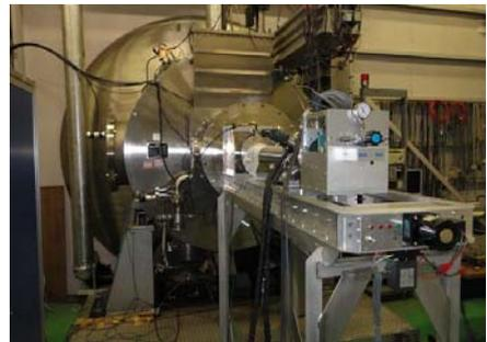
**Figure 4. The 3 m diameter vacuum chamber for the ion engine test.**
