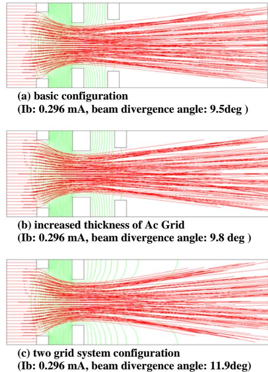
**Figure 10. Ion beam trajectory in condition of  $V_a/V_b=1,000/-500 \text{ V}$ ,  $L=0.8 \text{ mm}$**
