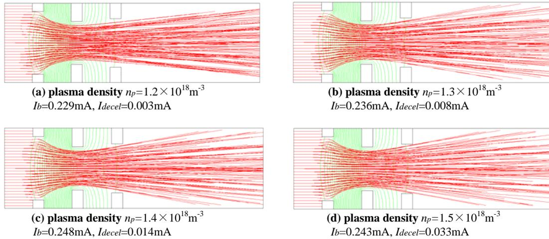
**Figure 9. Ion beam trajectory in condition of  $V_b/V_a=1,000/-400 \text{ V}$ ,  $L=1.0 \text{ mm}$**
