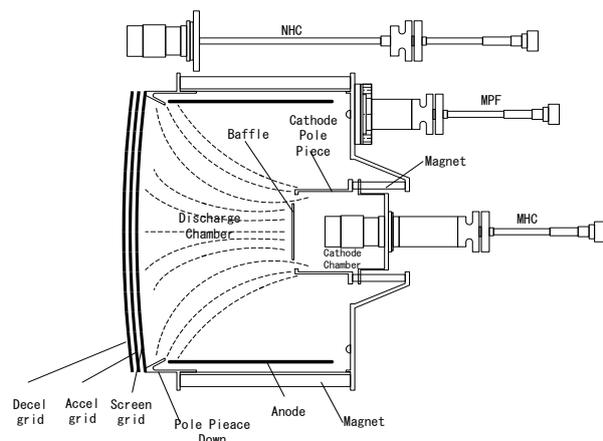
Figure 2. Schematic diagram of the thruster
