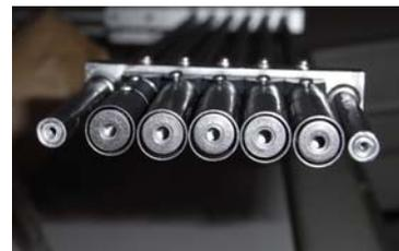
**Figure 5. Faraday probe for ion beam measurement**
