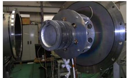
**Figure 3. The thruster attached to a boom with a flange.**
