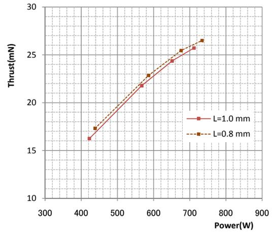
**Figure 7. The performance of power versus thrust.  $V_b/V_a=1,000/-500$  V**
