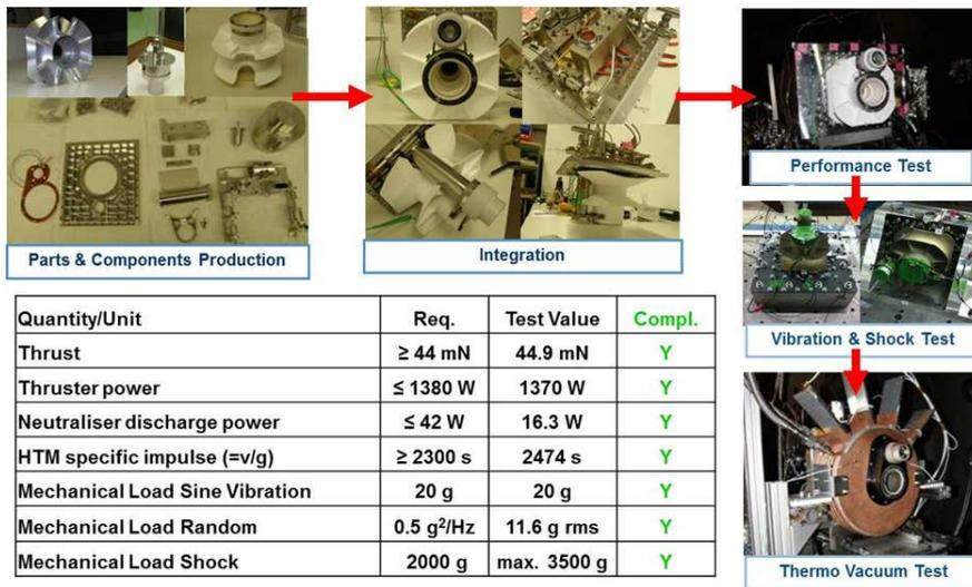
Figure 4: Photographs of the HEMPT Module EQM and performance verification table.
