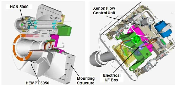
**Figure 3: 3D-drawing of the HEMPT Module.**
