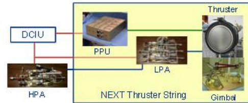
**Figure 1. NEXT Ion Propulsion System Components**
