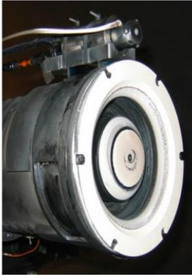
**Figure 6. Photograph of the NASA-103M.XL thruster after 4,731 hours of testing at 700 V.**
