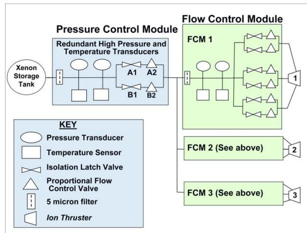
Figure 11. Advanced Xenon Feed System Configuration
