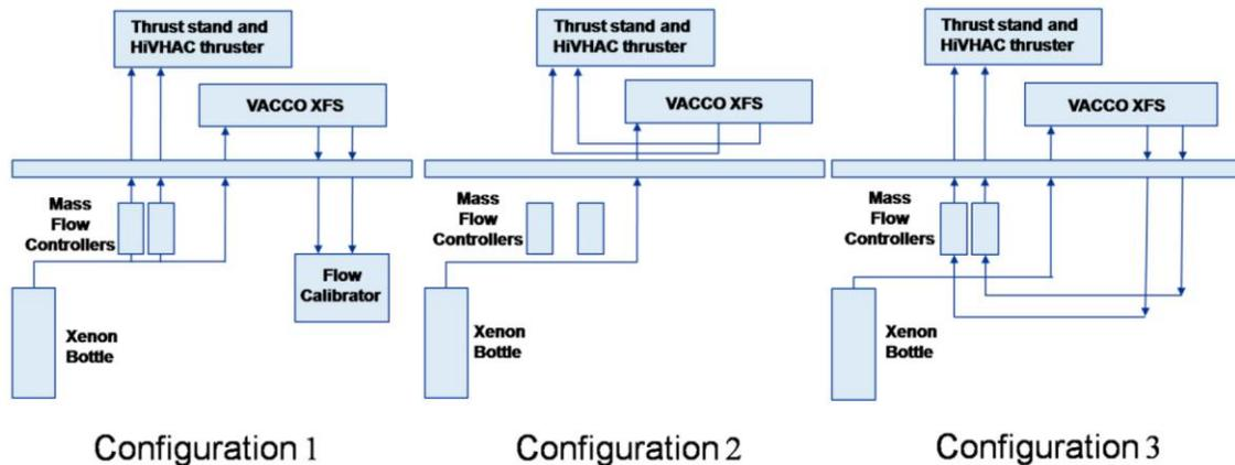
**Figure 13. Testing configurations of the AXFS.**
