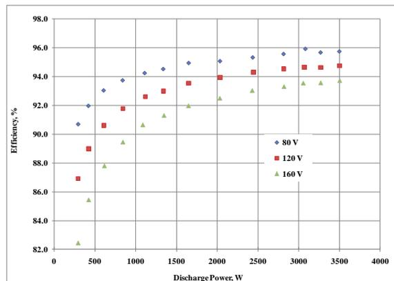
**Figure 10. Discharge power supply module efficiency at various input voltages.**
