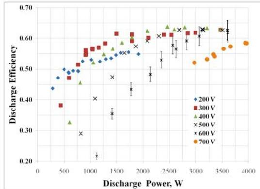
**Figure 8. HIVHAC EM discharge efficiency vs. discharge power for discharge voltage operation between 200 and 700 volts.**
