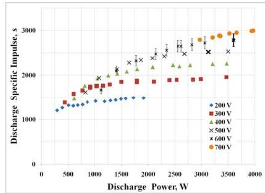
**Figure 9. HIVHAC EM discharge specific impulse vs. operating power for discharge voltage operation between 200 and 700 V.**
