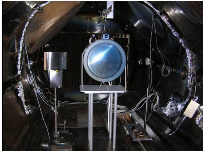
**Figure 5. Photograph of NEXT thruster installed in The Aerospace Corporation vacuum facility.**
