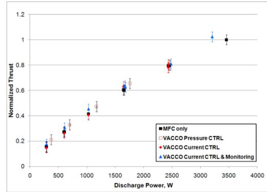
Figure 14. Performance characterization of Hall thruster with various XFS configurations.
