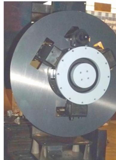
**Figure 7. HIVHAC EM-R thruster installed in VF12.**
