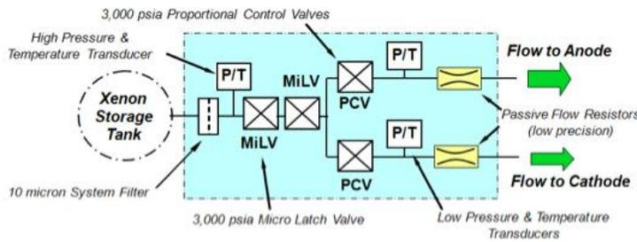
Figure 15. Hall Module XFCM schematic
