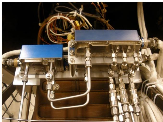
Figure 12. AXFS mounted on the HIVHAC thrust stand.
